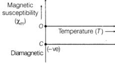
This is the graph for variation of  $\chi_m$  with temperature (T) of diamagnetic substance for material B.
